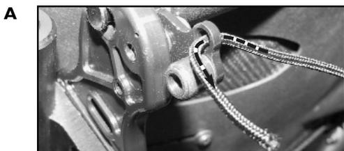
Thread cord through the latch mechanism.
